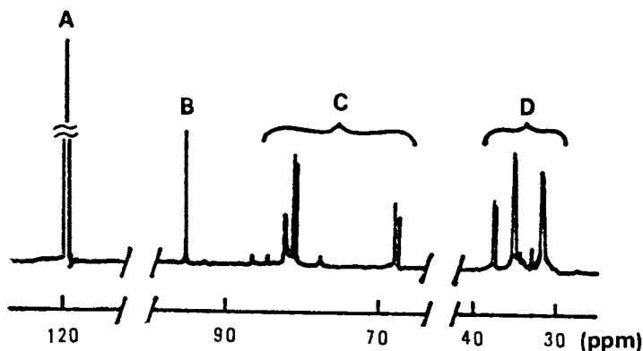
Figure 3. ^{31}\text{P} \{^1\text{H}\} NMR spectrum of the MeI-initiated polymerization of 2 after 490 min at 35^\circ\text{C} in \text{CH}_3\text{CN} . [\text{M}]_0 = 1.0 mol/L and [\text{I}]_0 = 0.20 mol/L.
